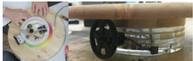
Figure 5: The Gadgeteer configuration underneath the Lazy Susan. When one turntable is turned, the remote ‘other’ turntable rotates to a matching position on the color gradient.
